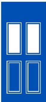
2F Mid Panel Cut out: 236 x 579mm Glass: 207 x 550mm
