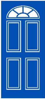
9V Sunburst Cut out: R292 x 279mm Glass: R279 x 254mm
