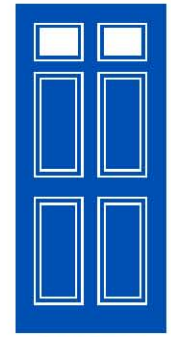
9S Twin Tops Cut out: 229 x 181mm Glass: 202 x 154mm
