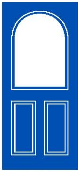
7A Half Glazed Arch Top Cut out: 585 x 940mm Glass: 558 x 912mm
