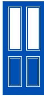
9N Twin Vertical Cut out: 229 x 940mm Glass: 203 x 912mm
