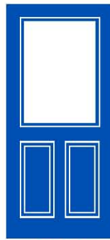
9Q Half Glazed Cut out: 585 x 940mm Glass: 558 x 912mm
