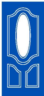
9X Oval Cut out: 451 x 1017mm Glass: 426 x 991mm
