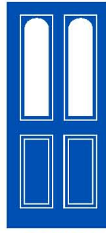
7D Twin Arch (rectangular glass) Cut out: 229 x 940mm Glass: 203 x 912mm
