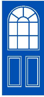
7B Half Glazed Arch Top with grid Cut out: 585 x 940mm Glass: 558 x 912mm
